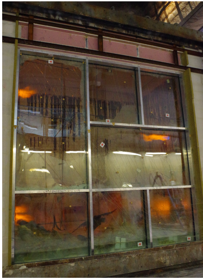
Fig. 22. Unexposed side of the test specimen, t = 6 m
