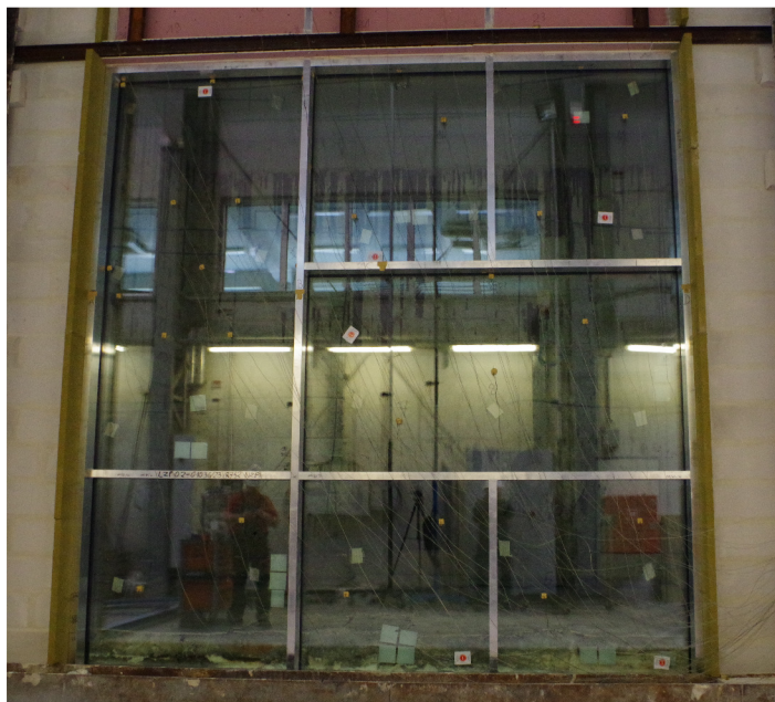
Fig. 2. Test specimen before the test - unexposed side
