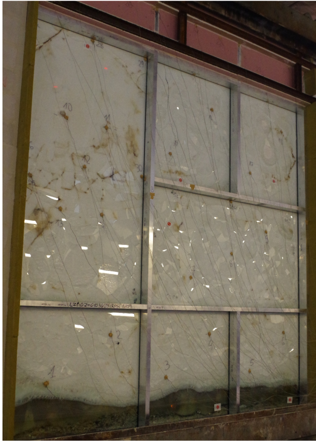
Fig. 24. Unexposed side of the test specimen, t = 46 m
