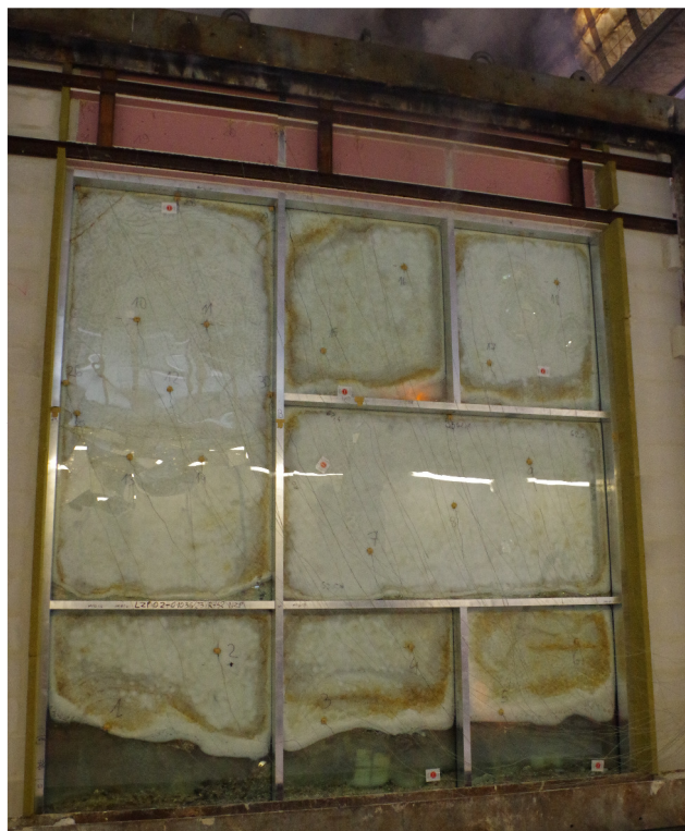
Fig. 23. Unexposed side of the test specimen, t = 21 m
