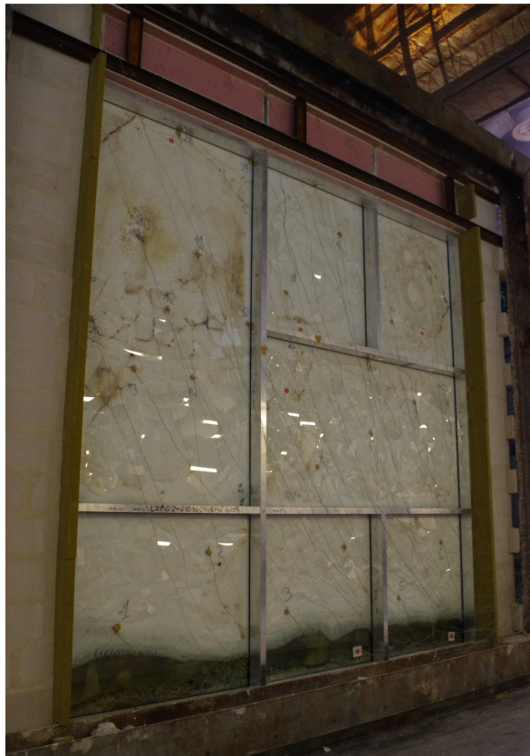
Fig. 25. Unexposed side of the test specimen after the test
