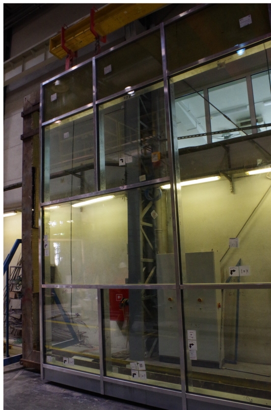
Fig. 1. Test specimen before the test – exposed side (before facing the furnace)
